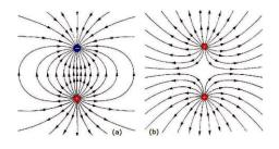
2. Consider the interaction between two charged particles. The lines of force shows the direction of 'electric filed'.
